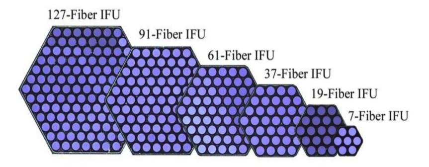
Figure 1. Photographs of MaNGA IFUs, ranging from the largest IFU (127 fibers, left) to the mini-bundle used for standard star observations (7 fibers, right). Individual fibers deviate with an RMS of only 3  $\mu$ m from an ideal hexagonal packing. Image taken from Drory et al. (2015).
